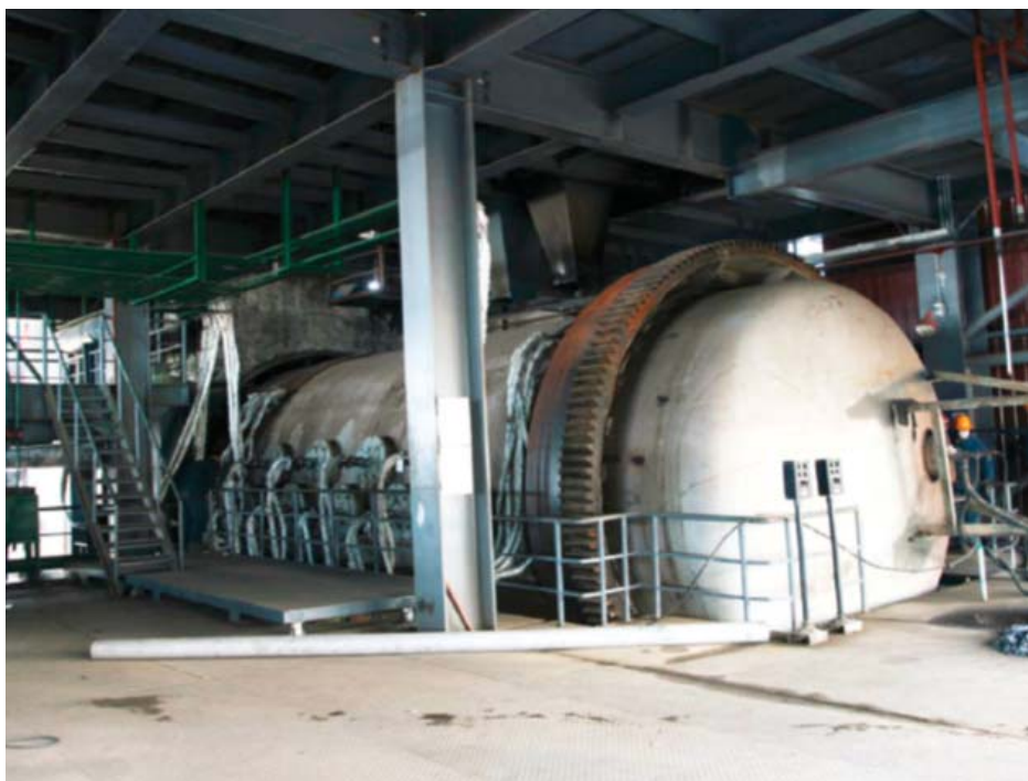
Figure 7 – The SKS reactor vessel ( 4.4 m diameter by 16.5 m long) at the Dongying copper smelter in China.
